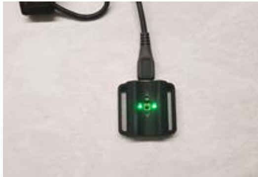
Figure 1. "Fingerbeeper" device that utilizes green photodiode as a light source.
